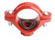
Caution: Piping practices require that main and branch connections are at a true 90° angle. Also be certain that the locating collar is securely positioned inside the outlet hole before tightening the housing. When mechanical tees or mechanical crosses are used as transition pieces between two runs, the tees or crosses shall be assembled prior to making the branch connections.
