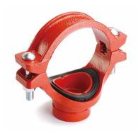
Caution: Piping practices require that main and branch connections are at a true 90° angle. Also be certain that the locating collar is securely positioned inside the outlet hole before tightening the housing. When mechanical tees or mechanical crosses are used as transition pieces between two runs, the tees or crosses shall be assembled prior to making the branch connections.
